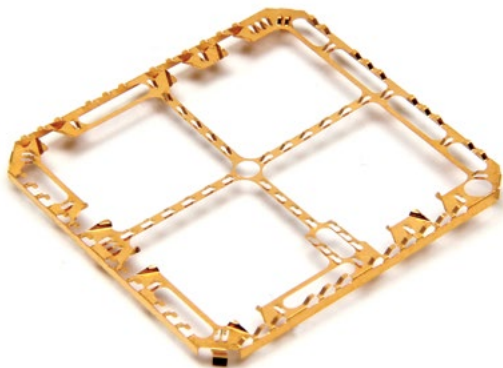
.003" Thick Beryllium Copper RFI Shield. Photoetched Blank. Die Formed. Heat Treated. Gold Plated
