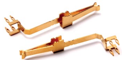
.012" Thick Beryllium Copper Contact Springs. Photoetched Blank. Die Formed. Heat Treated. Gold Plated.
